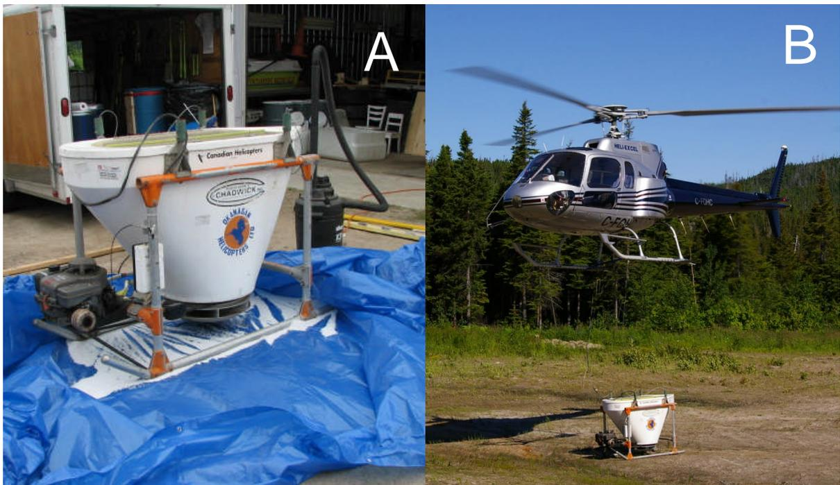
**Figure 2.** Equipment used for the dry application of the pheromone flakes. A) the spreader; B) The helicopter under which was attached the spreader.
